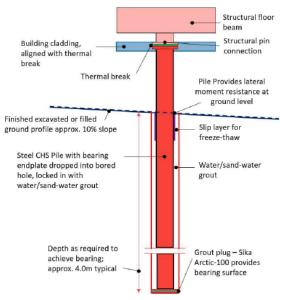
Figure 33: Sketch of the proposed end-bearing pile.
