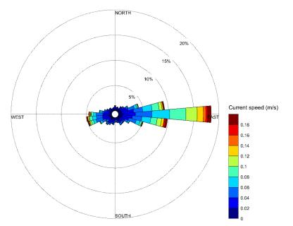
Figure 91. Current speed and direction at SB1 during November 2019. Distribution of depth-averaged current direction (degrees True) and velocity (m/s) between 28/10 and 18/11/19<sup>33</sup>.
