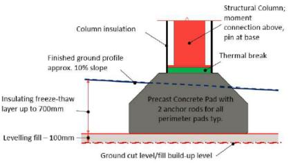
Figure 63: Diagram illustrating the proposed pad foundation option.
