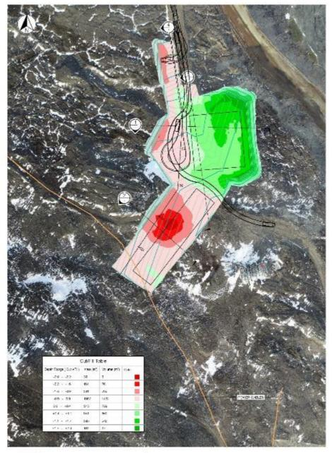
Figure 41: Preliminary temporary Scott Base Area A earthworks requirements.
