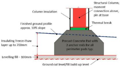
Figure 42: Pad foundations proposed for the temporary base buildings.
