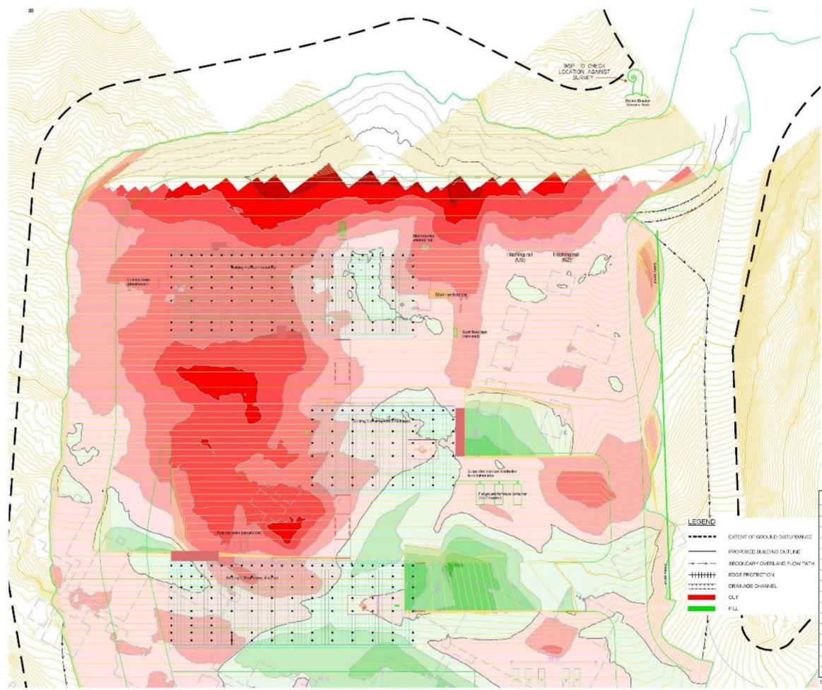
Figure 29: Detail of bulk earthworks plan with pile locations for the proposed Scott Base buildings (WSP, 2020).
