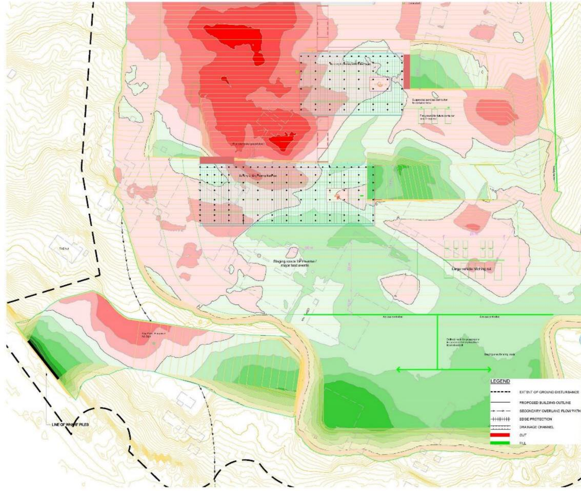
Figure 30: Detail of bulk earthworks with location of the wharf and the piling locations for Buildings B and C (WSP, 2020).
