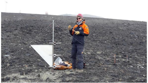
Figure 107: An MWAC dust sampler being installed at one of the monitoring sites behind the current Scott Base. Photo: O'Neill, University of Waikato.
