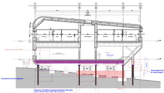
Figure 47: Side view of SPMTs delivering a building module to site. Red hash denotes the temporary platform due to gradient differences across the building platform.
