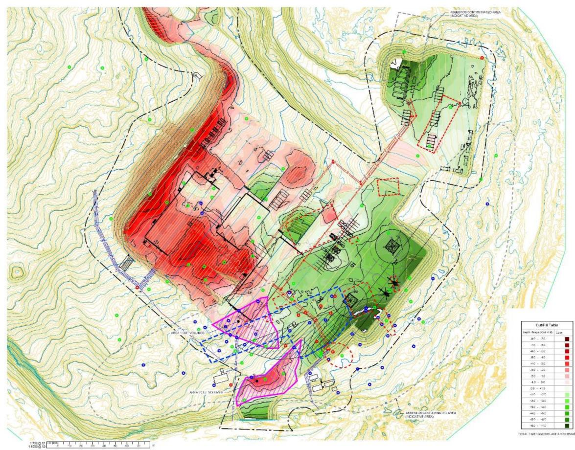
Figure 32: Plan showing the cut (red) and fill (green) profile with contamination areas both known and inferred superimposed (WSP, 2020).
