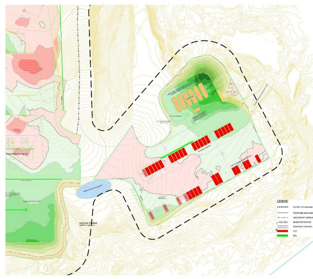
Figure 31: Detail of bulk earthworks with location of the proposed container line and bulk fuel storage. This is also the proposed staging location for construction equipment and the current buildings for removal (WSP, 2020).
