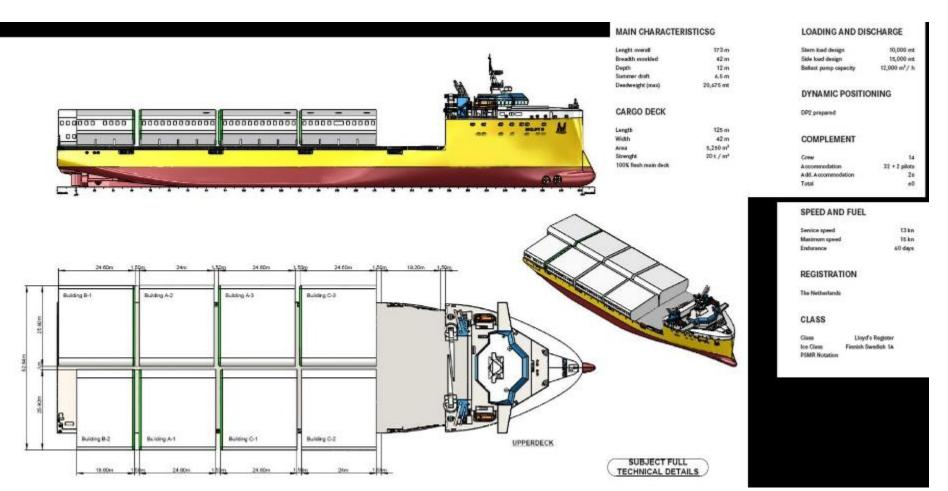
Figure 43: Preliminary loading arrangement and characteristics of the proposed MC Class vessel for the delivery of the building modules<sup>17</sup>.
