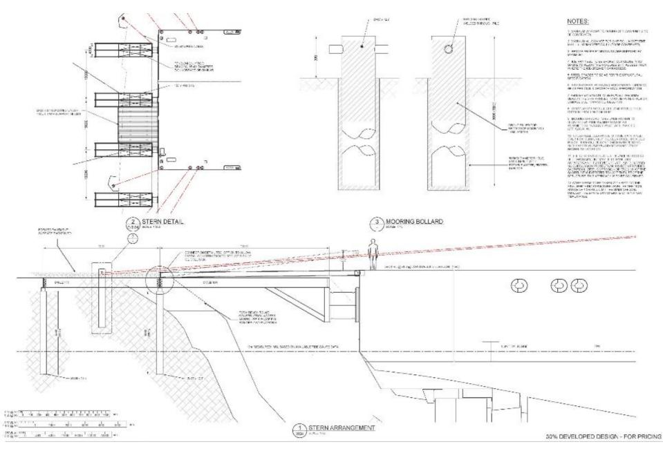
Figure 36: Plan view of the temporary wharf (top left), foundation pile and bollard detail (top right) and side view indicating the piles, cantilevered wharf, fender and ship.
