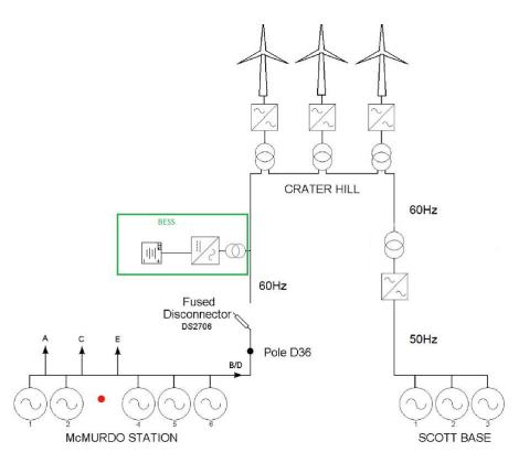
Figure 50: Power system concept design indicating from left to right, the McMurdo generators and distribution, the proposed BESS, proposed turbines, frequency converter, and Scott Base generators.
