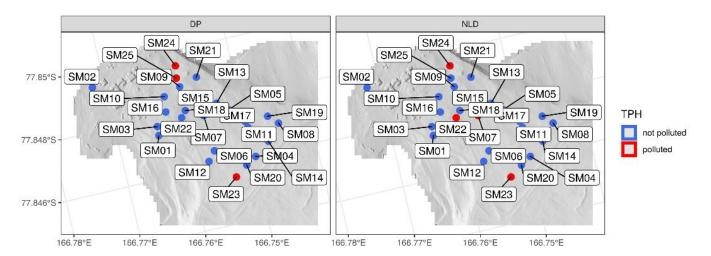
Figure 78: Estimated TPH contamination in surface soils (0-2cm) and soils at depth (2-10cm) at each of the soil monitoring sites above Scott Base.
