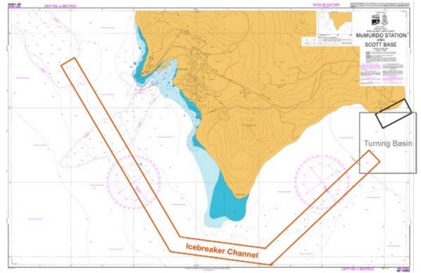
Figure 48: Indicative location of the additional icebreaker channel required to reach Pram Point.
