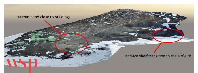
Figure 25: The Scott Base to McMurdo road is very close to Scott Base. (Base image: WSP, 2020)
