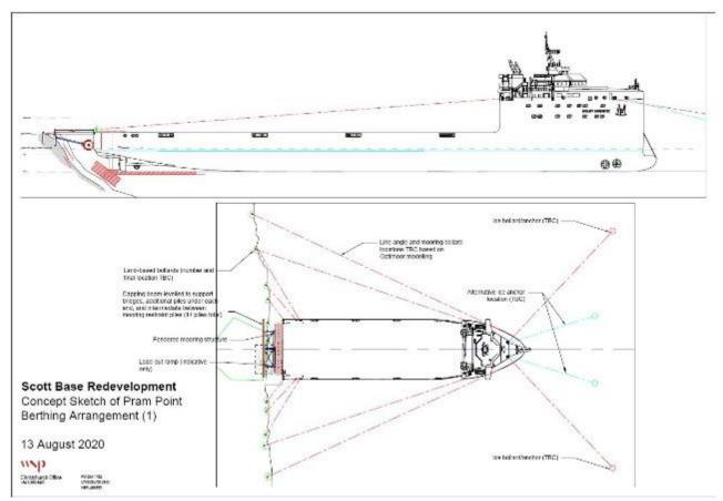
Figure 45: Plan and elevation view of the berthing arrangement.
