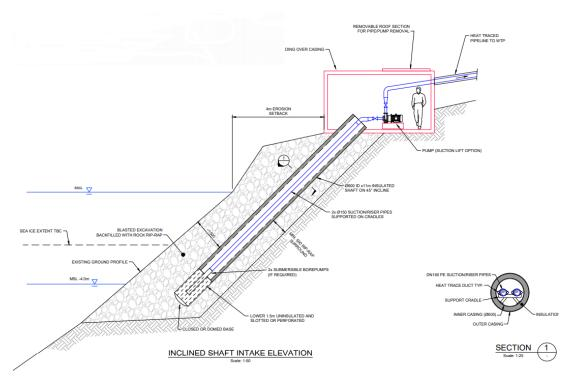
Figure 35: Concept view of water intake showing the cut channel, pipe lay and pump hut.
