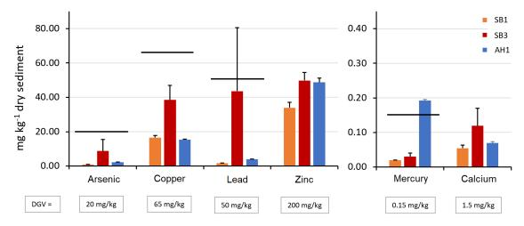
Figure 89. Sediment heavy metal contaminant concentrations at SB1, SB3 and AH1<sup>31</sup>.
