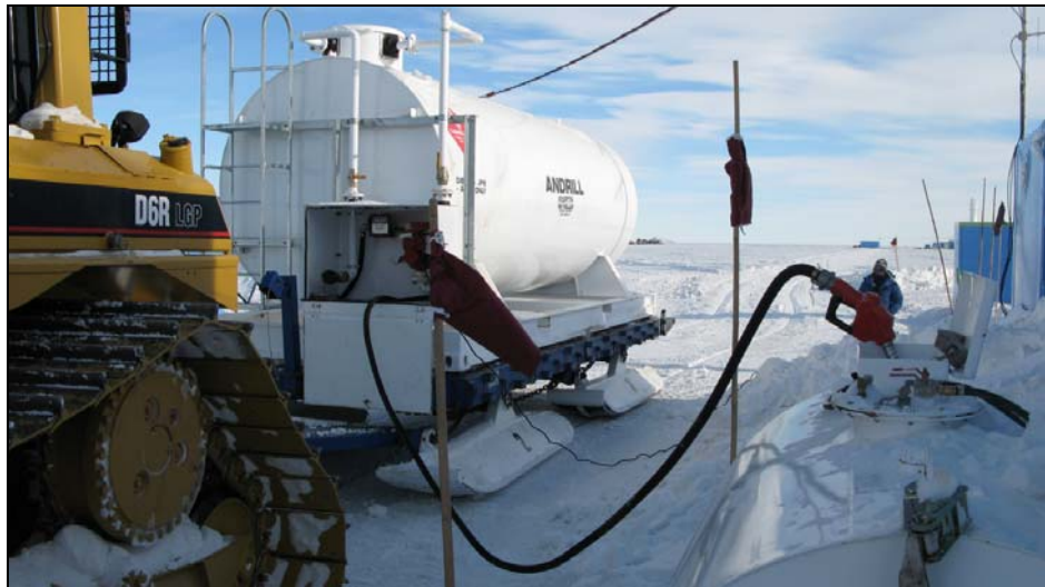
Figure 10. Refuelling from bulk to day tanks at ANDRILL SMS site
