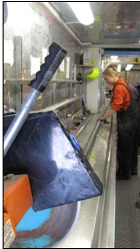
Figure 2. Cleaning and initial description of core at ANDRILL SMS site laboratory
