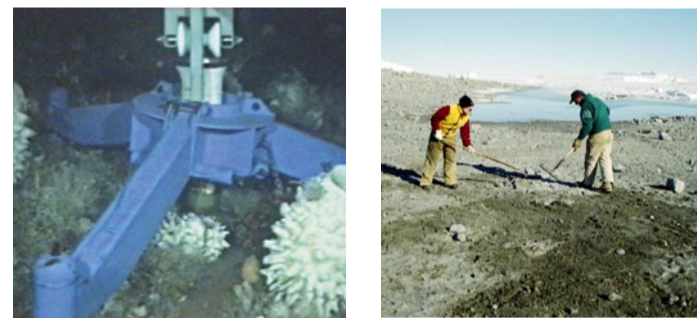
Figure 2: Left: An image taken from video monitoring of the first season of drilling, showing the sea riser guide base amongst siliceous sponges, a sea floor silica needle sponge mat and other benthic organisms. (Waterhouse, 2001). Right: Cape Roberts Project Manager and Camp Assistant raking to loosen compacted soil.
